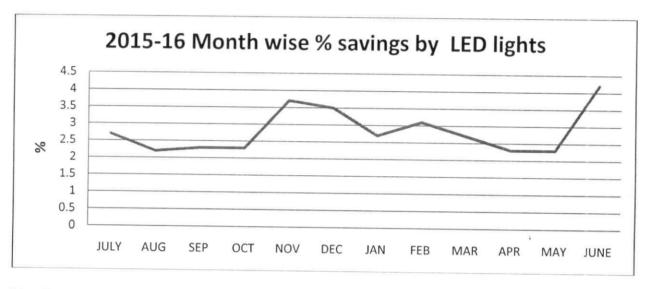
Month wise saving % in the campus for the duration of 2015-2016 is shown in Figure. The total savings of annual energy is 47972 Kwh or units. It is observed that the % savings improvement up to 4.2 % in the month of June.
