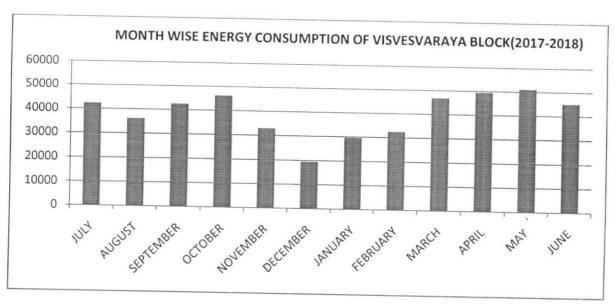
The monthly wise power consumption of the VISVESVARAYA BLOCK for the duration of 2017-2018 is shown in Figure. The total annual energy consumption during 2017-18 is 474373 Kwh or units. Peak consumption is observed in the month of May with 51102 units. The average monthly consumption for VISVESVARAYA BLOCK recorded is 39531 units.
