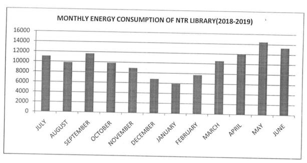
The monthly wise power consumption of the NTR LIBRAY for the duration of 2018-2019 is shown in Figure. The total annual energy consumption v during 2018-19 is 122159 Kwh or units. Peak consumption is observed in the month of May with 14467 units. The average monthly consumption for NTR LIBRARY recorded is 10179 units.
