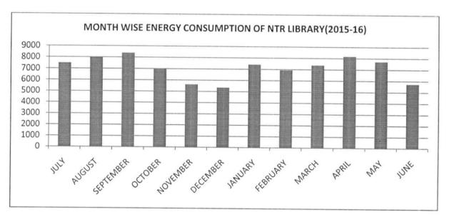
The monthly wise power consumption of the NTR LIBRAY for the duration of 2015-2016 is shown in Figure. The total annual energy consumption during 2019-20 is 85278 Kwh or units. Peak consumption is observed in the month of September with 8391 units. The average monthly consumption for NTR LIBRARY recorded is 7106 units.
