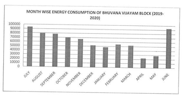
The monthly wise power consumption of the BHUVANA VIJAYAM BLOCK for the duration of 2019-2020 is shown in Figure. The total annual energy consumption during 2019-20 is 741476 Kwh or units. Peak consumption is observed in the month of July with 94181 units. The average monthly consumption for BHUVANA VIJAYAM BLOCK recorded is 61790 units.
