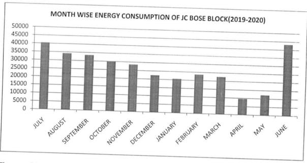
The monthly wise power consumption of the JC BOSE BLOCK for the duration of 2019-2020 is shown in Figure. The total annual energy consumption during 2019-20 is 321096 Kwh or units. Peak consumption is observed in the month of June with 43293 units. The average monthly consumption for JC BOSE BLOCK recorded is 26758 units.
