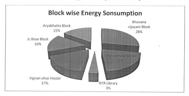
The block wise energy consumption of the university is shown in above Fig. The total annual energy consumption of the campus is 2446579 Kwh, of which 31% is from Bhuvana vijayam Block, 22% from Visvesvaraya Block, 14% from Aryabhatta Block, 15% from hostel, 14% from jc Bose blocl, 4% from library. The highest energy consumption is obtained from Bhuvan vijayam Block followed by different blocks in the campus.
