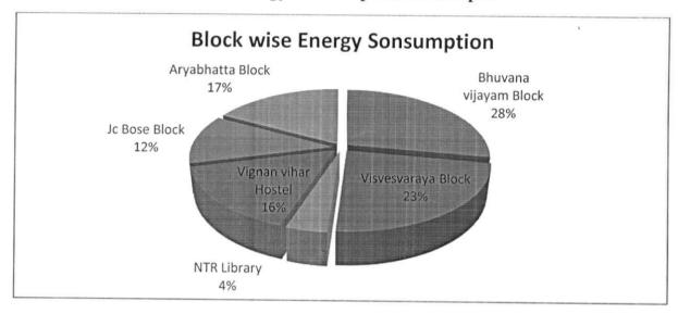
The block wise energy consumption of the university is shown in above Fig. The total annual energy consumption of the campus is 2048046 Kwh, of which 28% is from Bhuvana vijayam Block, 23% from Visvesvaraya Block, 17% from Aryabhatta Block, 16% from hostel, 12% from jc Bose blocl, 4% from library. The highest energy consumption is obtained from Bhuvan vijayam Block followed by different blocks in the campus.
