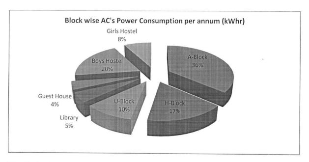
The block wise power consumption by ACs is shown in above figure. 36 % of energy consumption is from A-Block, 15% of energy consumption is from H-Block, 10 % of energy consumption is from U-Block, 20% of energy consumption is from boy's hostels, 8% of energy consumption is from Girls hostel, 4% of energy consumption is from guest house, 5% of energy consumption is from library. The highest energy consumption is obtained in A-Block followed by different blocks in the campus.
