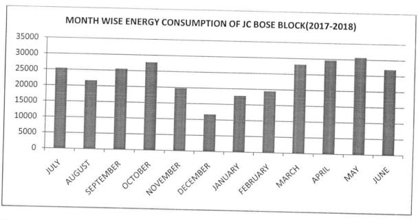
The monthly wise power consumption of the JC BOSE BLOCK for the duration of 2017-2018 is shown in Figure. The total annual energy consumption during 2017-18 is 284620 Kwh or units. Peak consumption is observed in the month of MAY with 30661 units. The average monthly consumption for JC BOSE BLOCK recorded is 23718 units.
