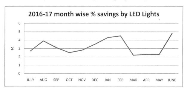
Month wise saving % in the campus for the duration of 2016-2017 is shown in Figure. The total savings of annual energy is 50479 Kwh or units. It is observed that the % savings improvement up to 4.8 % in the month of June.
