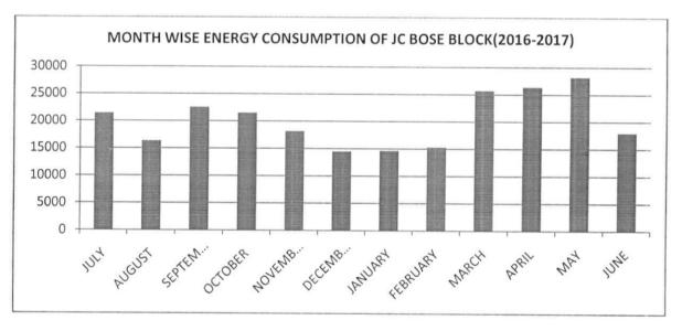
The monthly wise power consumption of the JC BOSE BLOCK for the duration of 2016-2017 is shown in Figure. The total annual energy consumption during 2016-17 is 242675 units. Peak consumption is observed in the month of MAY with 28239 units. The average monthly consumption for JC BOSE BLOCK recorded is 20222 units.
