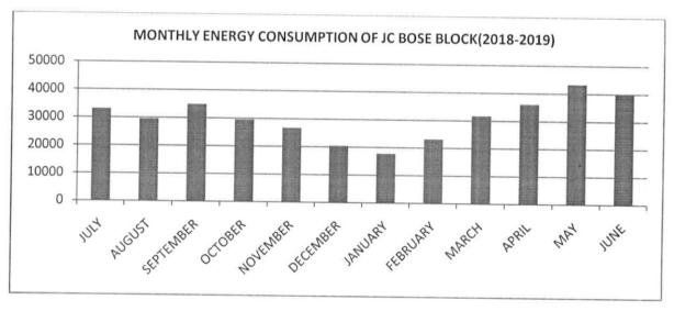
The monthly wise power consumption of the JC BOSE BLOCK for the duration of 2018-2019 is shown in Figure. The total annual energy consumption during 2018-19 is 366488 Kwh or units. Peak consumption is observed in the month of MAY with 43404 units. The average monthly consumption for JC BOSE BLOCK recorded is 30540 units.
