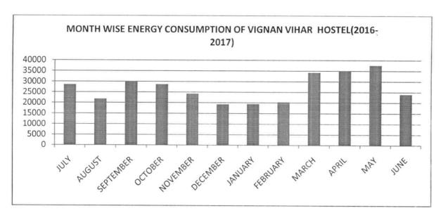
The monthly wise power consumption of the VIGNAN VIHAR HOSTEL for the duration of 2016-2017 is shown in Figure. The total annual energy consumption during 2016-17 is 323568 Kwh or units. Peak consumption is observed in the month of May with 37652 units. The average monthly consumption for VIGNAN VIHAR HOSTEL recorded is 26964 units.
