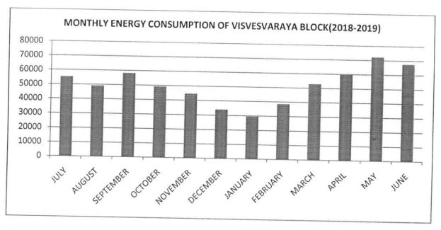
The monthly wise power consumption of the VISVESVARAYA BLOCK for the duration of 2018-2019 is shown in Figure. The total annual energy consumption during 2018-19 is 611788 Kwh or units. Peak consumption is observed in the month of May with 72339 units. The average monthly consumption for VISVESVARAYA BLOCK recorded is 50982 #nits.
