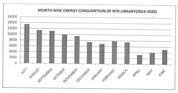
The monthly wise power consumption of the NTR LIBRARY for the duration of 2019-2020 is shown in Figure. The total annual energy consumption during 2019-20 is 97647 Kwh or units. Peak consumption is observed in the month of July with 13454 units. The average monthly consumption for NTR LIBRARY recorded is 8137 units.
