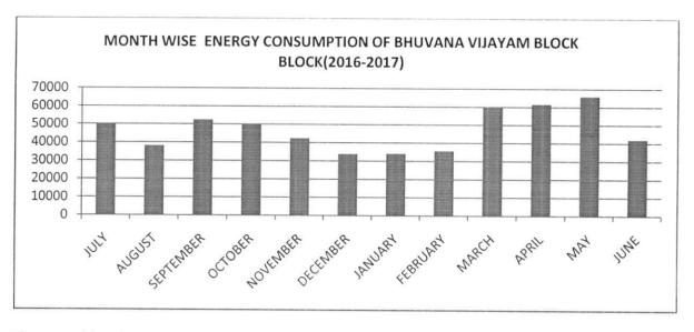
The monthly wise power consumption of the BHUVANA VIJAYAM BLOCK for the duration of 2016-2017 is shown in Figure. The total annual energy consumption during 2016-17 is 566246 Kwh or units. Peak consumption is observed in the month of May with 65891 units. The average monthly consumption for BHUVANA VIJAYAM BLOCK recorded is 47187 units.
