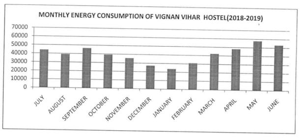
The monthly wise power consumption of the VIGNAN VIHAR HOSTEL for the duration of 2018-2019 is shown in Figure. The total annual energy consumption during 2018-19 is 488654 Kwh or units. Peak consumption is observed in the month of May with 57871 units. The average monthly consumption for VIGNAN VIHAR HOSTEL recorded is 40721 units.
