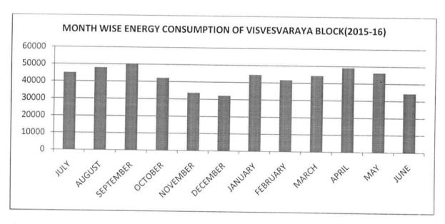
The monthly wise power consumption of the VISVESVARAYA BLOCK for the duration of 2015-2016 is shown in Figure. The total annual energy consumption during 2019-20 is 511701 Kwh or units. Peak consumption is observed in the month of September with 50349 units. The average monthly consumption for VISVESVARAYA BLOCK recorded is 42641 units.
