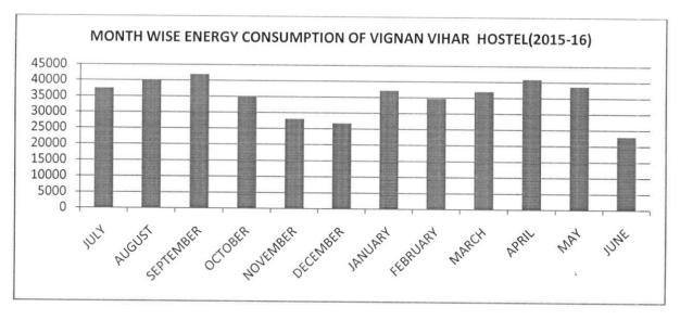
The monthly wise power consumption of the VIGNAN VIHAR HOSTEL for the duration of 2015-2016 is shown in Figure. The total annual energy consumption during 2019-20 is 420686 Kwh or units. Peak consumption is observed in the month of September with 41958 units. The average monthly consumption for VIGNAN VIHAR HOSTEL recorded is 35057 units.
