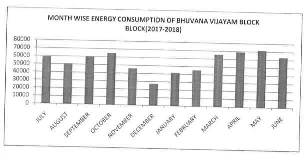
The monthly wise power consumption of the BHUVANA VIJAYAM BLOCK for the duration of 2017-2018 is shown in Figure. The total annual energy consumption during 2017-18 is 664125 Kwh or units. Peak consumption is observed in the month of May with 71545 units. The average monthly consumption for BHUVANA VIJAYAM BLOCK recorded is 55343 units.
