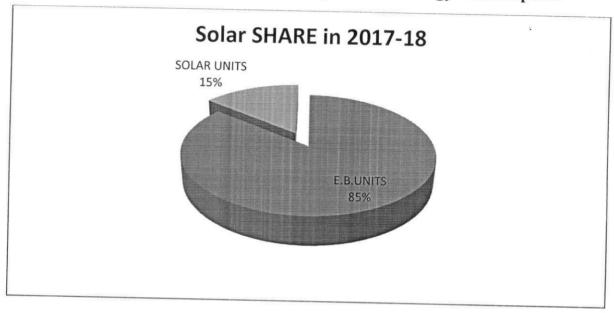
The modes of energy utilisation in VFSTR campus is shown in Figure. The diagram shows the VFSTR utilises 15 % of energy from 1MW solar PV plant and 85% energy from grid supply.
