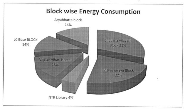
The block wise energy consumption of the university is shown in above Fig. The total annual energy consumption of the campus is 2414770 Kwh, of which 31% is from Bhuvana vijayam Block, 22% from Visvesvaraya Block, 14% from Aryabhatta Block, 15% from hostel, 14% from jc Bose blocl, 4% from library. The highest energy consumption is obtained from Bhuvan vijayam Block followed by different blocks in the campus.
