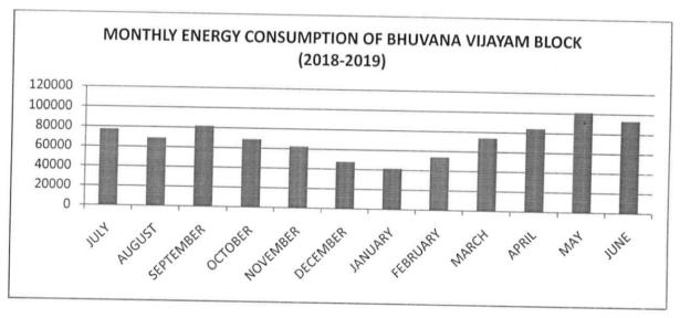
The monthly wise power consumption of the BHUVANA VIJAYAM BLOCK for the duration of 2018-2019 is shown in Figure. The total annual energy consumption during 2018-19 is 855145 Kwh or units. Peak consumption is observed in the month of May with 101275 units. The average monthly consumption for BHUVANA VIJAYAM BLOCK recorded is 71262 units.
