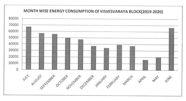
The monthly wise power consumption of the VISVESVARAYA BLOCK for the duration of 2019-2020 is shown in Figure. The total annual energy consumption during 2019-20 is 529625 Kwh or units. Peak consumption is observed in the month of July with 67272 units. The average monthly consumption for VISVESVARAYA BLOCK recorded is 44135 units.
