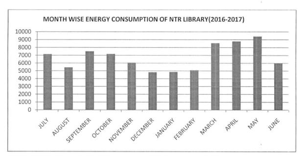
The monthly wise power consumption of the NTR LIBRAY for the duration of 2016-2017 is shown in Figure. The total annual energy consumption during 2016-17 is 80888 Kwh or units. Peak consumption is observed in the month of May with 9413 units. The average monthly consumption for NTR LIBRARY recorded is 6740 units.
