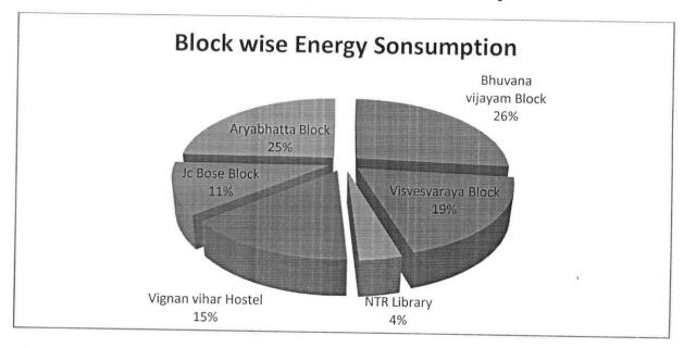
The block wise energy power consumption of the university is shown in above Fig. The total annual energy consumption of the campus is 2521323 Kwh, of which 26% is from Bhuvana vijayam Block, 19% from Visvesvaraya Block, 25 % from Aryabhatta Block, 15 % from hostel, 11% from jc Bose blocl, 4% from library. The highest energy consumption is obtained from Bhuvan vijayam Block followed by different blocks in the campus
