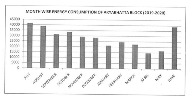
The monthly wise power consumption of the ARYABHATTA BLOCK for the duration of 2019-2020 is shown in Figure. The total annual energy consumption during 2019-20 is 341227 Kwh or units. Peak consumption is observed in the month of July with 41363 units. The average monthly consumption for ARYABHATTA BLOCK recorded is 28435 units.
