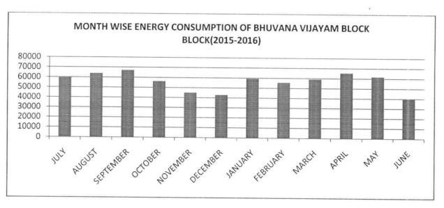
The monthly wise power consumption of the BHUVANA VIJAYAM BLOCK for the duration of 2015-2016 is shown in Figure. The total annual energy consumption during 2019-20 is 676538 Kwh or units. Peak consumption is observed in the month of September with 67132 units. The average monthly consumption for BHUVANA VIJAYAM BLOCK recorded is 56378 units.
