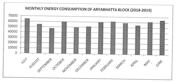
The monthly wise power consumption of the ARYABHATTA BLOCK for the duration of 2018-2019 is shown in Figure. The total annual energy consumption during 2018-19 is 690369 Kwh or units. Peak consumption is observed in the month of July with 65158 units. The average monthly consumption for ARYABHATTA BLOCK recorded is 57530 units.
