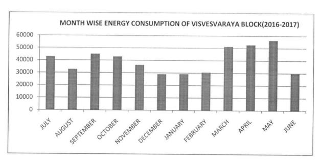
The monthly wise power consumption of the VISVESVARAYA BLOCK for the duration of 2016-2017 is shown in Figure. The total annual energy consumption during 2016-17 is 479359 Kwh or units. Peak consumption is observed in the month of May with 56478 units. The average monthly consumption for VISVESVARAYA BLOCK recorded is 399946 units
