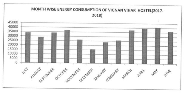
The monthly wise power consumption of the VIGNAN VIHAR HOSTEL for the duration of 2017-2018 is shown in Figure. The total annual energy consumption during 2017-18 is 379497 Kwh or units. Peak consumption is observed in the month of May with 40882 units. The average monthly consumption for VIGNAN VIHAR HOSTEL recorded is 31624units.
