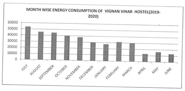
The monthly wise power consumption of the VIGNAN VIHAR HOSTEL for the duration of 2019-2020 is shown in Figure. The total annual energy consumption during 2019-20 is 383699 Kwh or units. Peak consumption is observed in the month of July with 53817 units. The average monthly consumption for VIGNAN VIHAR HOSTEL recorded is 31974 units.
